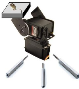
Figure 11 - Shows two stepper motors linked with a bracket, connected to the bottom of the animal bed (Trossen, 2006).
