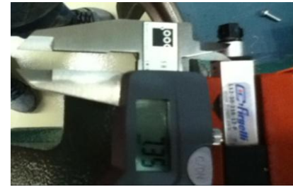
Figure 18 – Measuring the starting position of 20% with the digital caliper.
