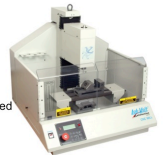
Figure 10: Local prototyping company, Tosa Tool, has CNC milling with 0.007 mm. precision http://www.tosatool.com/askaboutproducts/fut9600-cnc-milling.jpg
