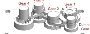
Figure 4: A full rotation of a long gear leads to a partial rotation of a shorter gear, thus allowing the disks to rotate in increments rather than continuously
