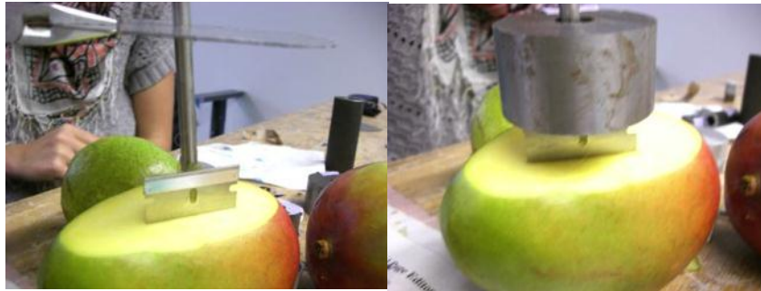
Figure 12: Cutting Force test without weight (left) and with weight added (right)
