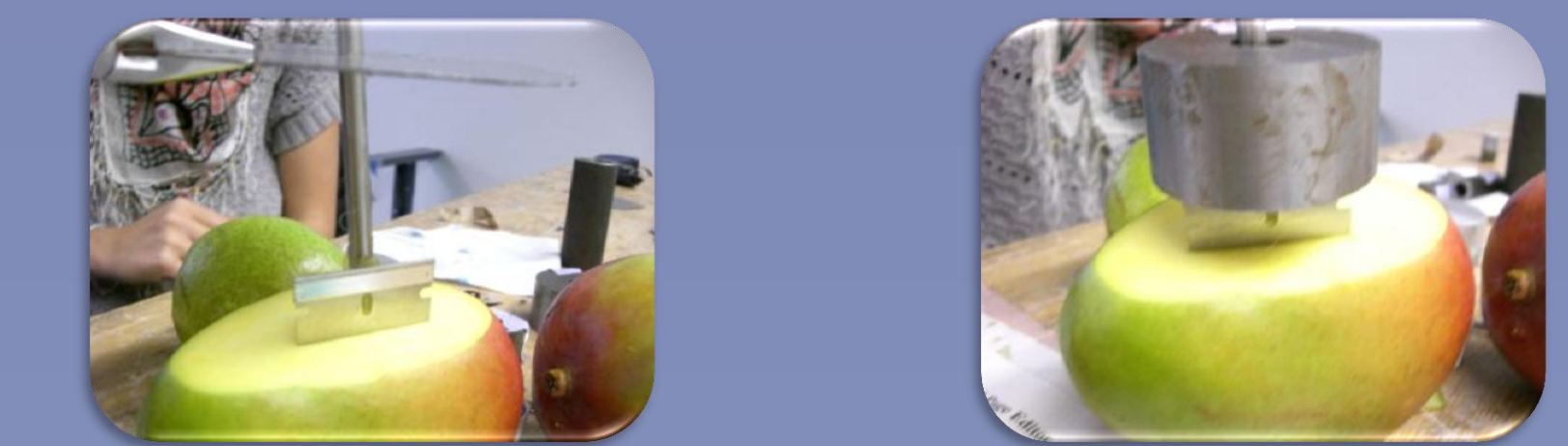
Figure 11. Setup of Cutting Force test without weight (left) and with weight added (right)
