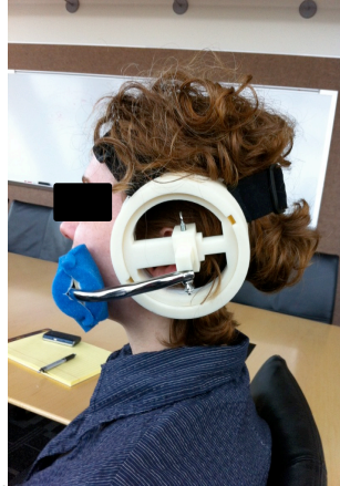
Figure 14. Rapid prototype of complete headgear device tested on the team’s client.
