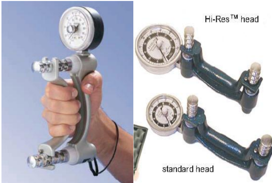
Figure 1. Two commonly used hand dynamometers. Figure 1.1 shows the Jamar model, while Figure 1.2 shows the Baseline model. The Baseline model is slightly less expensive than the Jamar model. Figures from http://www.thehumansolution.com/jahady.html .
