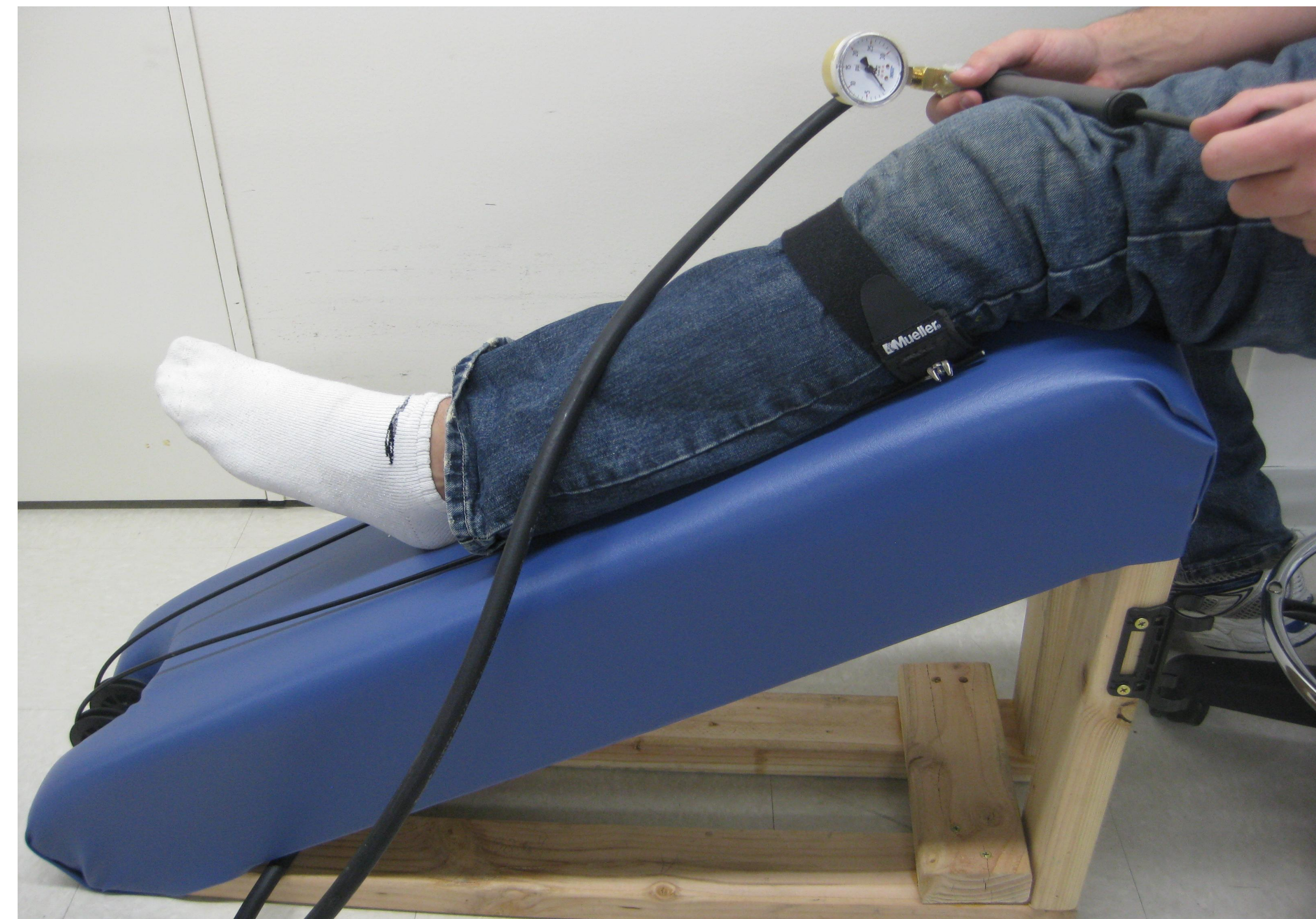
Figure 3: Overall structure of final design including vinyl fabric, two inch thick padding and triangular structure made of 2x4 wooden beams.
