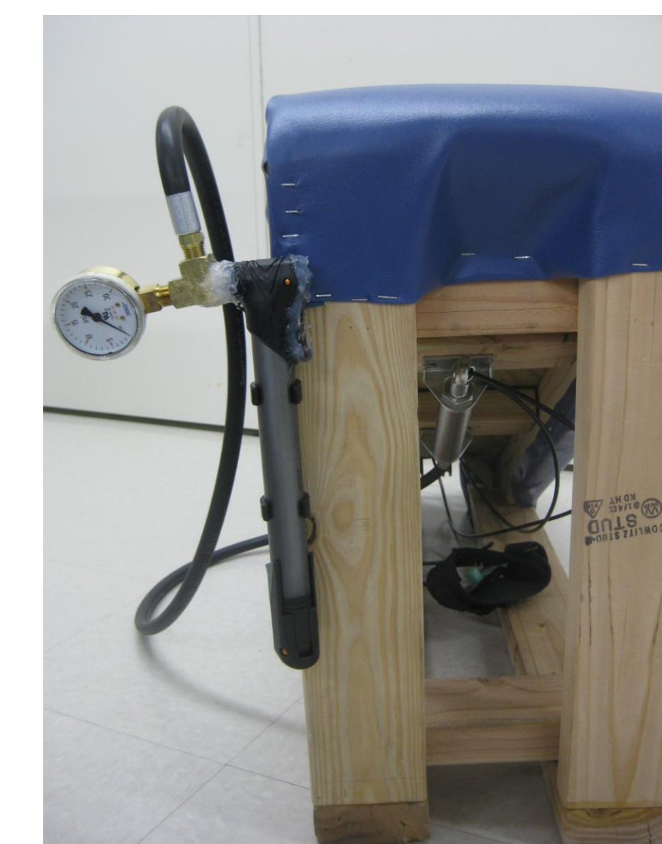
Figure 5: Back view of air cylinder with hose and wire attached.
