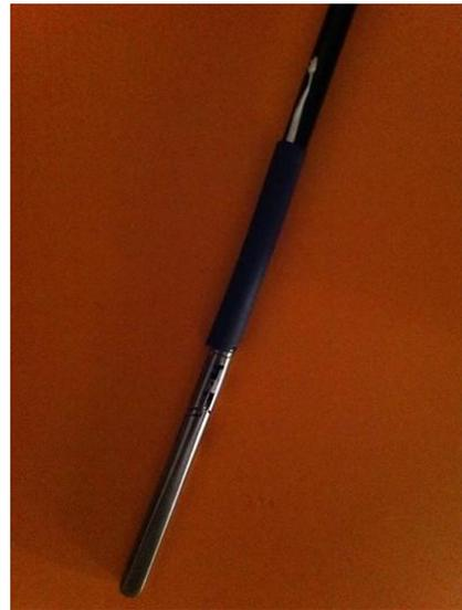
Figure 6: Close up of the Heat Shrink Wrap design.
