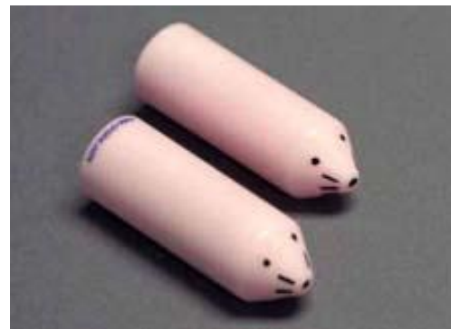
Figure 1. Water-filled mouse phantoms used primarily with CT scanners
