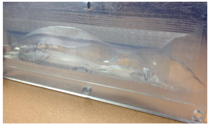
Figure 12. Half of the printed mold for the rat phantom
