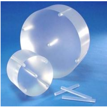
Figure 2. Circular phantoms used to test CT dosage 4
