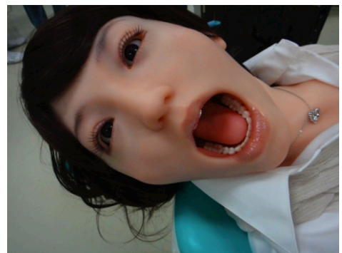
Figure 1: The Showa Hanko 2 robotic dental test dummy.
