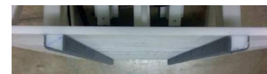
Figure 5 – Base tracking composed of HDPE cut at a 11.5° angle with yoga mat padding
