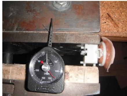
Figure 17. Force testing set-up. The prosthesis was placed in a vice and the force meter was attached to the cords and pulled to create tension on the cords.
