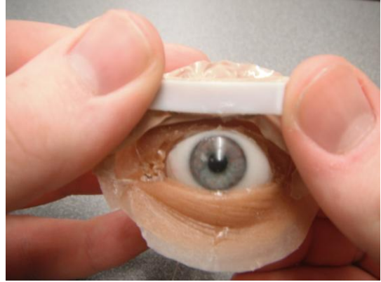
Figure 15. The eyelid with the strip of Teflon. The Teflon dramatically reduces the necessary force to move the eyelid.
