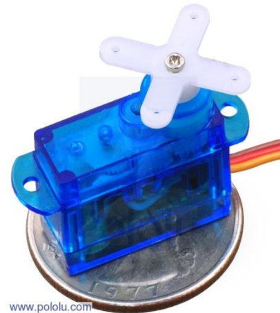
Figure 7. A comparison of a servo motor to a quarter. Servo motors can be very small and still provide relatively high torque. [12]
