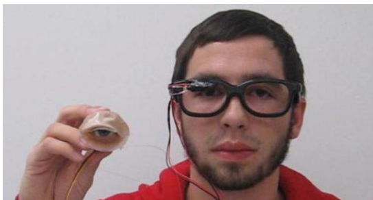
Figure 6. Current blinking prosthesis prototype. [7]
