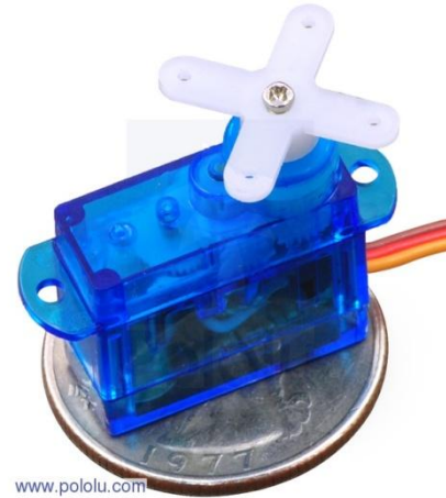
www.pololu.com Figure 7. A comparison of a servo motor to a quarter. Servo motors can be very small and still provide relatively high torque. [12]
