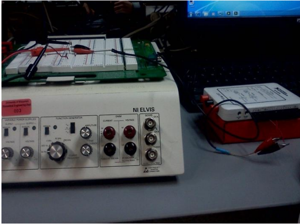
Figure 1: Velocity profiling set-up with the breadboard with resistor and reed switch on the
