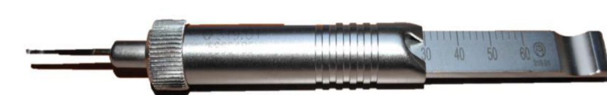
Figure 3: The depth gauge. Elimination of the need for this tool will save the orthopedic surgeon time during most of his surgeries.
