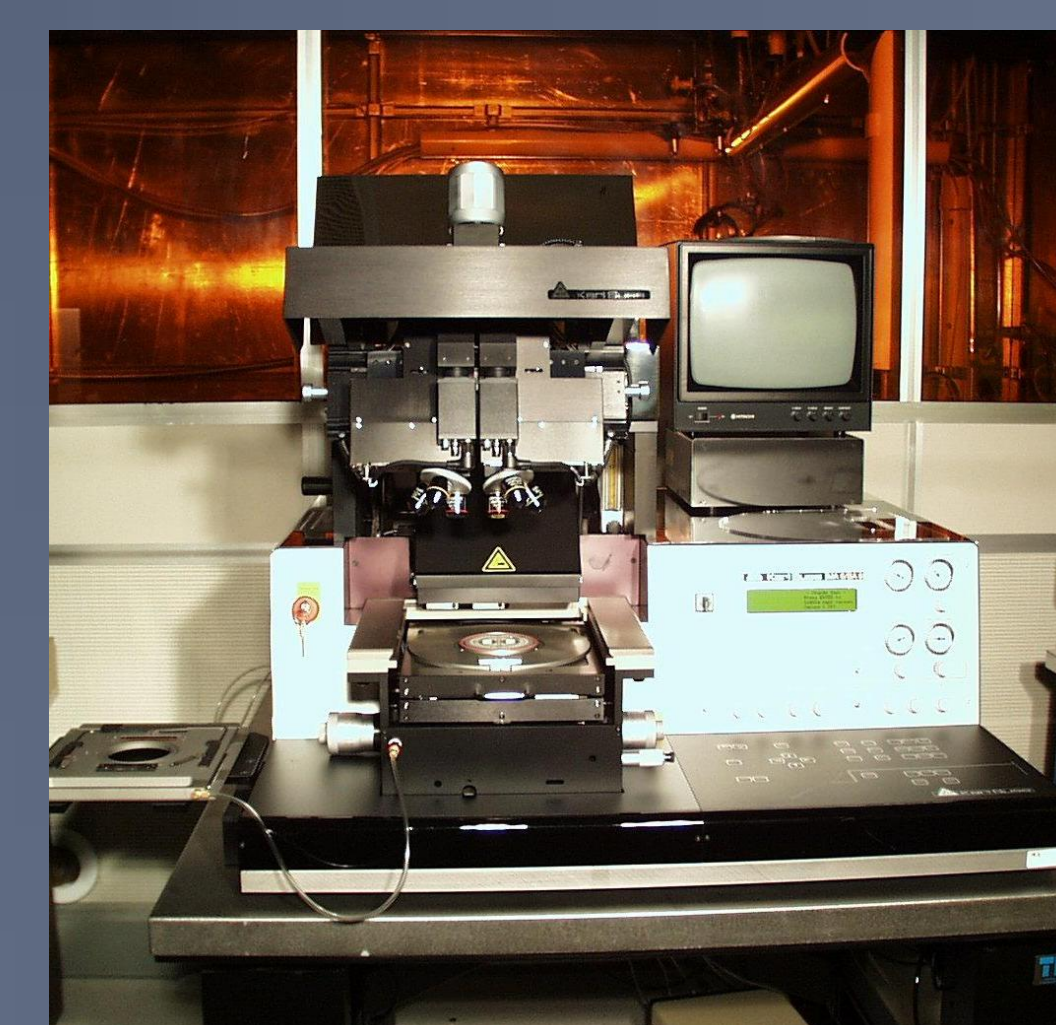
Figure 1: Karl Suss MA-6 used mask aligner [3]
