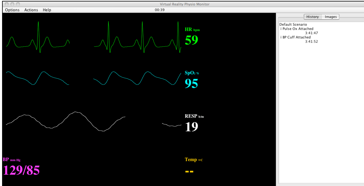
Figure 22: Vitals Monitor Final Design and User Interface. The sweeping bar updating the vitals is visible as a dark gap in the graphics. Blood pressure in mm Hg is displayed on the bottom left and the ECG, photoplethysmograph and respiration graphics and values in beats per minute, percent oxygen and breaths per minute are displayed respectively. The history log is displayed right above the monitor and the timer, options menu, actions menu and help menu are displayed above the monitor.
