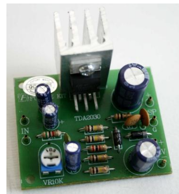
Figure 7: Example of a mono power amplifier Image Courtesy of: http://store.qkits.com/moreinfo.cfm/FA604
