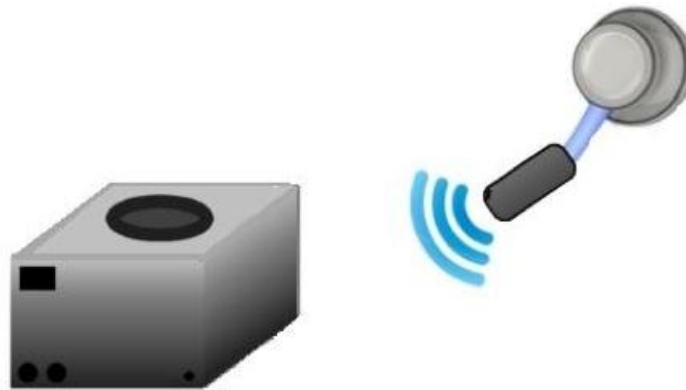
Figure 8: A depiction of the final design, featuring a main receiver box with a speaker, a headphone jack, and volume controls and one of the wireless microphones.
