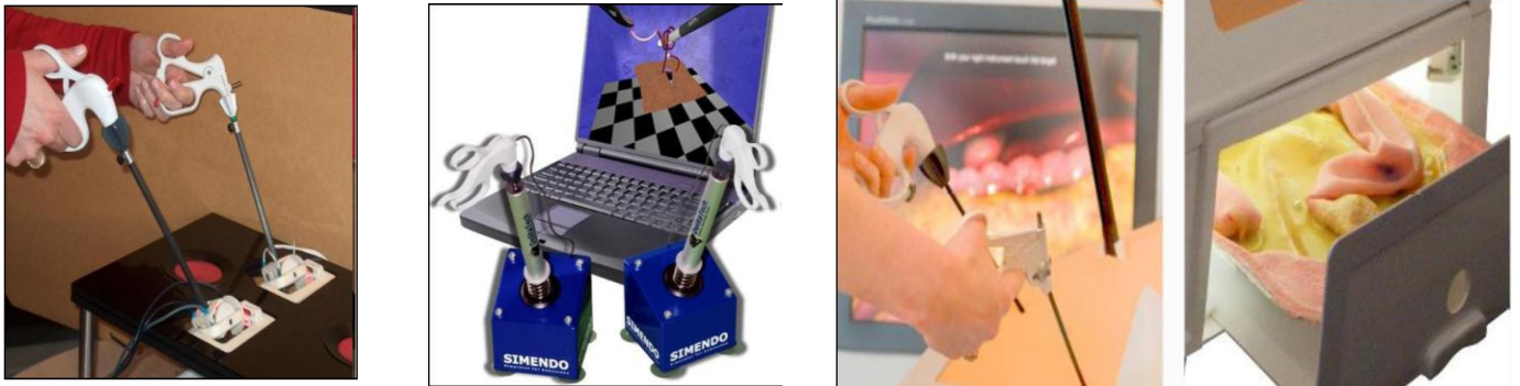
Figures 2-4: The TrEndo and SIMENDO surgical simulations (left and center) that incorporate the handheld instruments used to detect movement [5][6]. The ProMIS simulation (right) includes an anatomical model [7].
