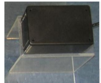
Figure 10: The new housing for the simplified circuit.
