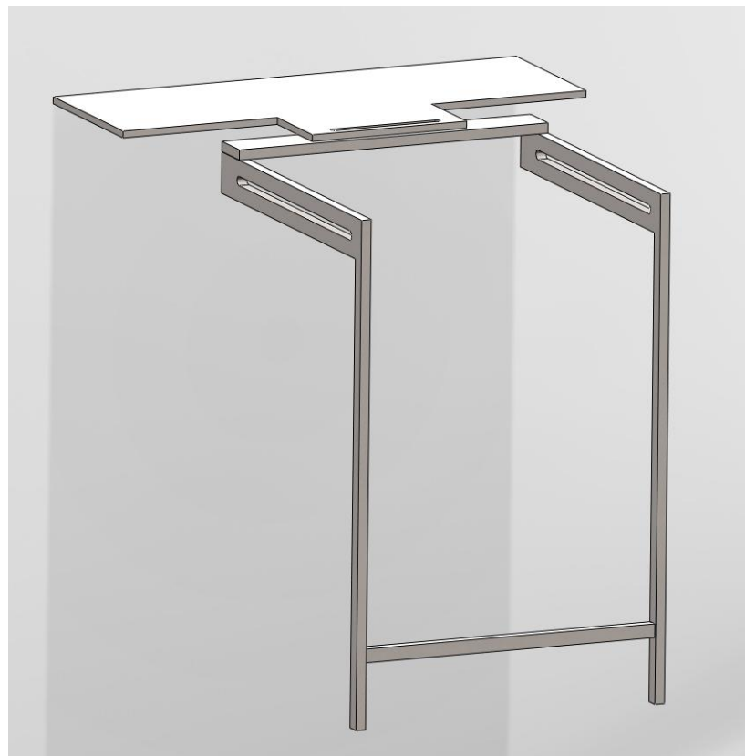
Figure 6: Bed Insert Design. The wide and flat part seen in the top of the picture is inserted under the mattress of the O.R. bed to support the device. A harness is attached to the slots in the top of the legs to support our client. SolidWorks design by Blake Marzella.
