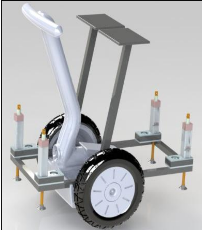
Figure 3. Segway LeanSeat Design to enable dynamic movement within the operating room
