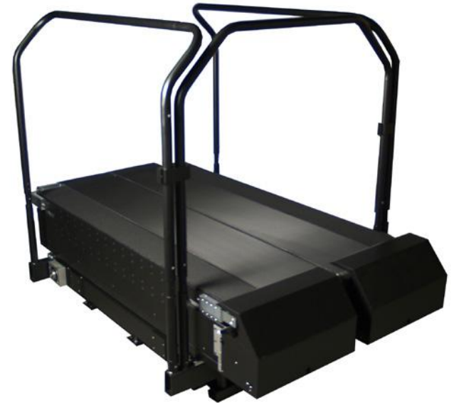
Figure 2. Treadmill instrumented with force plates.
