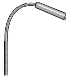
Figure 5: Goose-neck style used for the shaft of the clamp
