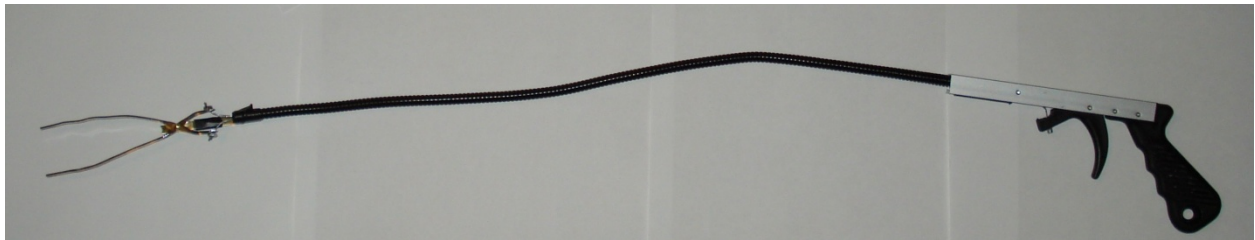
Figure 11: Final design incorporating the ratchet-style handle, the goose-neck shaft, and the curved clamp arms utilizing the bike brake mechanism to operate.
