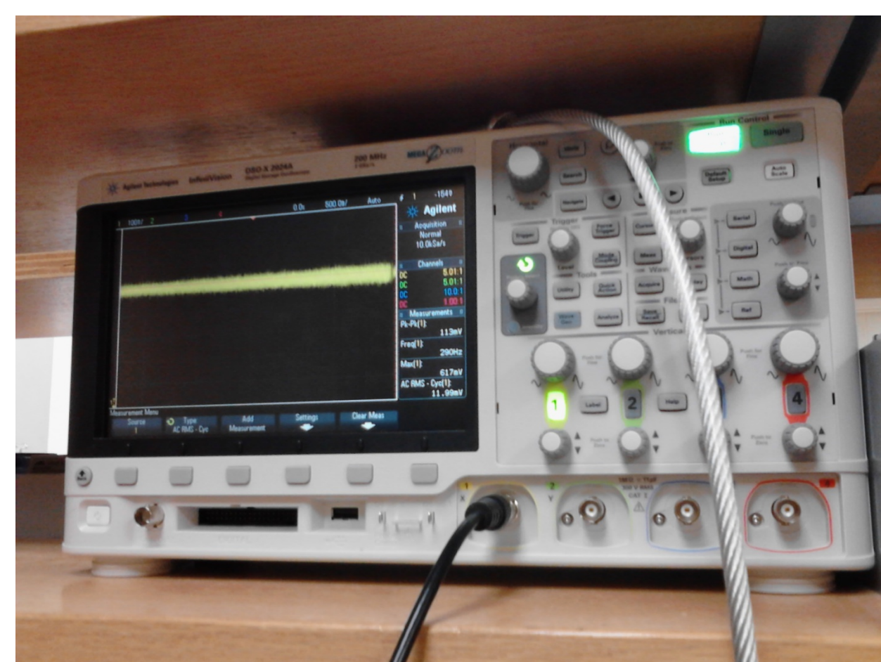
Figure 6. Increasing voltage signal on the oscilloscope as the transmitter moves closer to the antenna.
