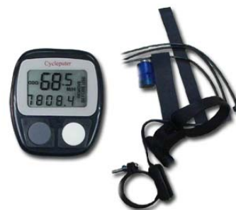
Figure 7: Bike speedometer with the equipment to count revolutions of a wheel. From http://image.made-in-china.com/2f0j00FeOEKtJhrRpj/Bicycle-Cycle-Computer.jpg
