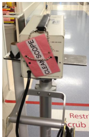
Figure 6: Current indication system used by UW-Hospital. Laminated paper sign displays “clean” on one side and “dirty” on the reverse side. These signs are unreliable and often neglected.
