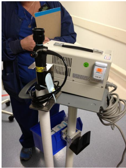
Figure 7: RFID tag mounted on a portable bronchoscope machine.
