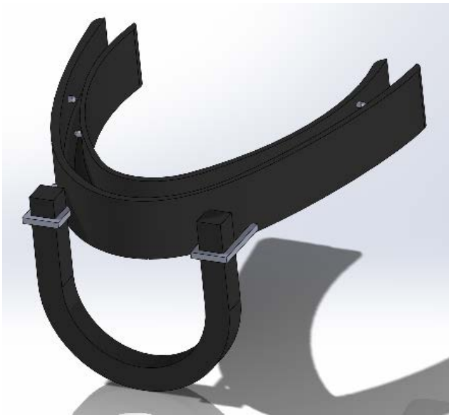
Figure 5: SolidWorks model of the fitted mouthpiece design depicting the pressure points in the mouthpiece and "U-shape" tube holder.
