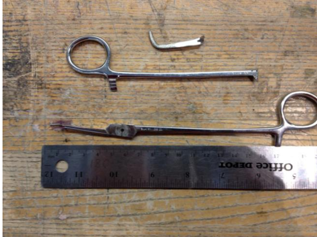
Figure 12: Completely dismantled right-angle forceps. The top arm was broken in the dismantling process.
