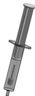
Figure 3: Syringe Hydrometer. Includes pre-calibrated counter weight, and syringe components. Liquid is pulled in the syringe and the internal component would
