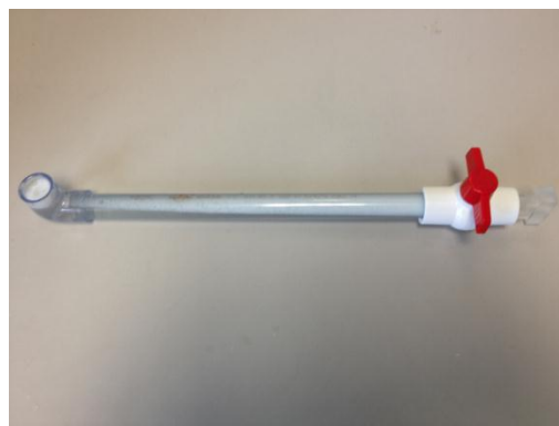
Figure 15: Adapter with soap solution within chamber lying prone to test adapter's effect on bubble propagation into the hydrometer. Observe bubbles residing across length of adapter.
