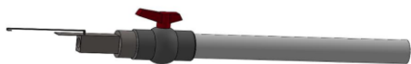
Figure 9: Design for the fish-tank hydrometer adapter utilizing a PVC pipe with a ball valve and the fabricated attachment piece. The extension (on the left side) would clip onto the hydrometer and block the hole on the side.
