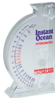
Figure 4: Commercially available fish tank hydrometer for specific gravity measurements.
