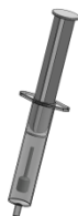
Figure 3: Syringe Hydrometer. Includes pre-calibrated counter weight, and syringe components. Liquid is pulled in the syringe and the internal component would float at levels depending on the density of the liquid.
