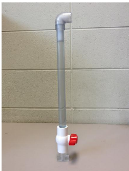
Figure 16: Adapter with soap solution tilted upwards. Observe bubbles no longer reside along the length of the adapter, rather at the top, and away from the hydrometer that would be situated beneath.
