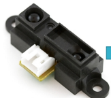
Figure 3: Sharp gp2y0a2xkf sensor. http://www.google.com/imgres?start=0&num=10&hl=en&safe=off&ibc=d&ibw
