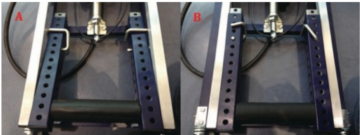
Figure 21: Illustration of how locking pin orientation affects collapsibility – (A) Pins inserted from the side of the tubing prohibits the device from folding; (B) Pins inserted from the front or back allow for collapsibility, but are susceptible to falling out when the device is folded.
