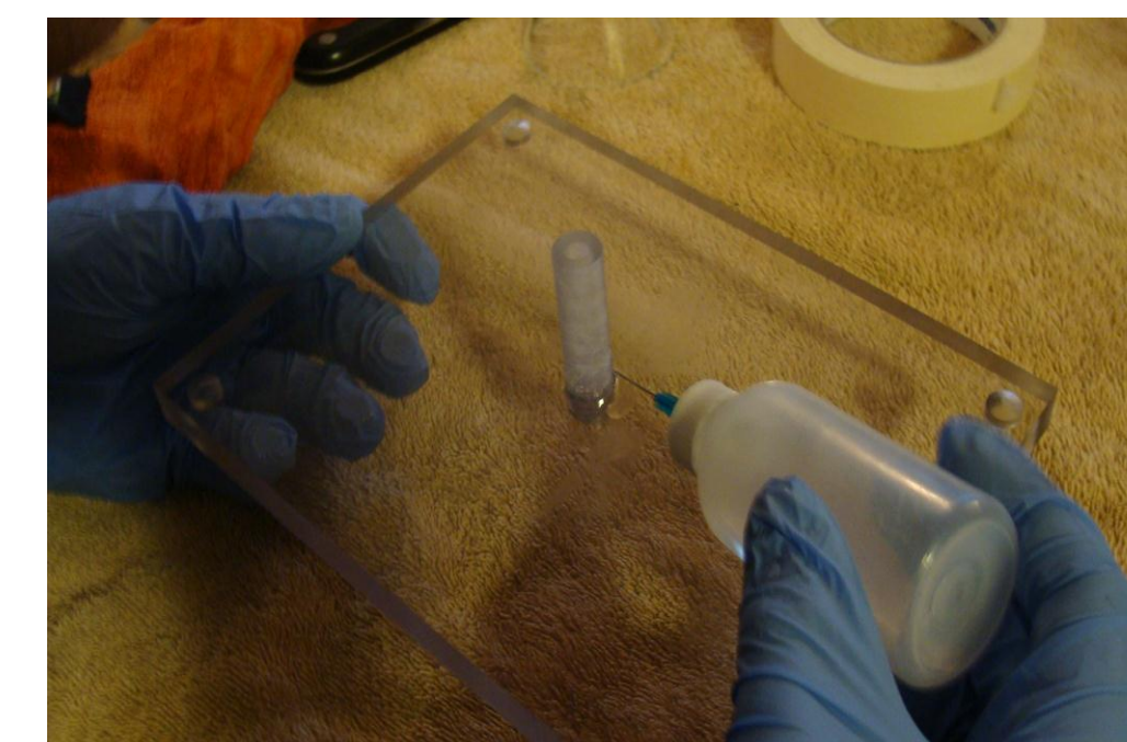
Figure 5: Gluing of fixed cylinder
