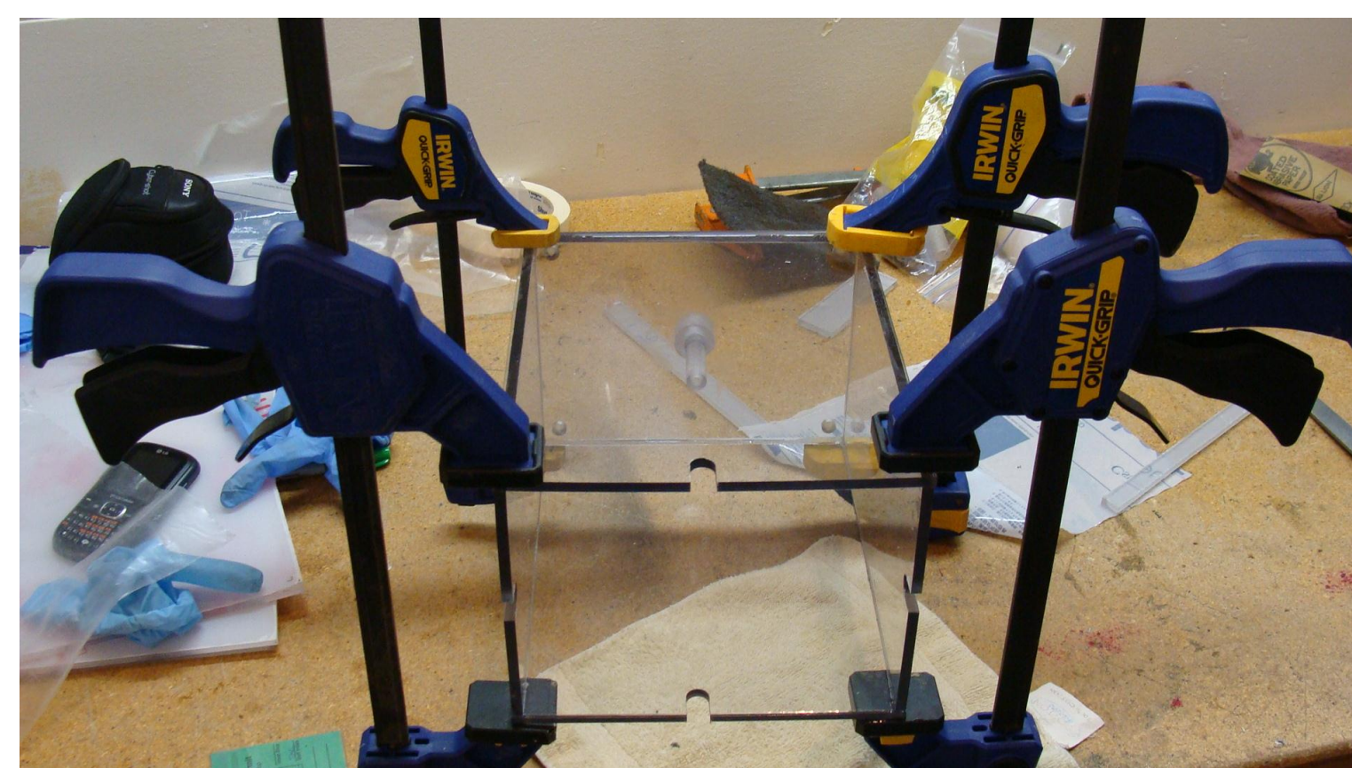
Figure 6: Cementing of outer walls
