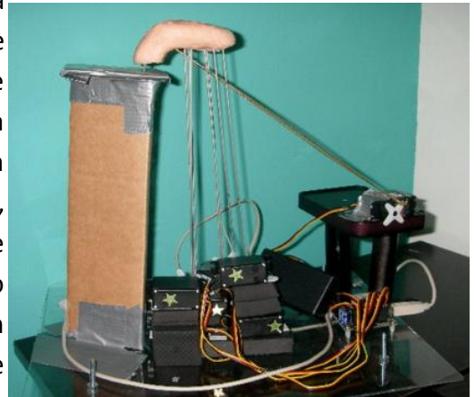
Figure 2: Previous Prototype - tongue constructed of silicone is moved with 8 rods that connect to 8 servos, cardboard base acts as support for tongue
