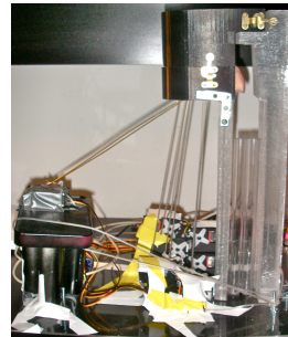
Figure 3: Image of the current prototype assembled with the hard palate, mandible, front support, and pharyngeal wall around the tongue.
