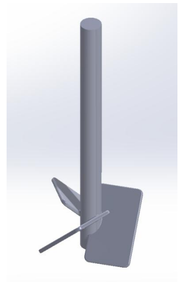
Figure 6: SolidWorks model of the pitched blade impeller. The dimensions of this design are shown in Figures B1, B2 in Appendix B.
