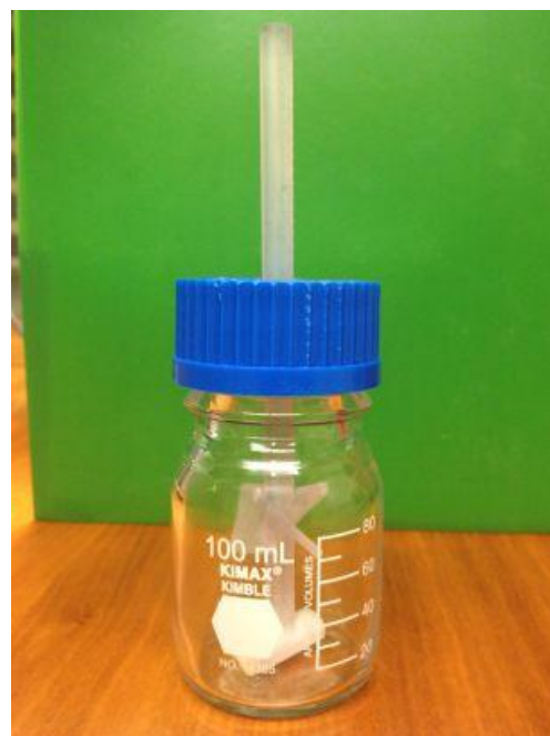
Figure 17: Photo of Accura60 impeller with magnetic stir bar in 100 mL bottle
