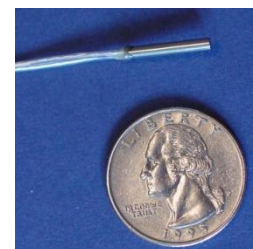
Figure 18: Image of a Miniature Pt100 RTD sensor [2].
