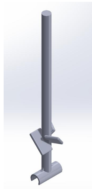
Figure 16. CAD model of the final impeller design. This CAD drawing was used to 3D print the part in Accura60. The dimensions are shown in Figures B6-B9 in Appendix B.
