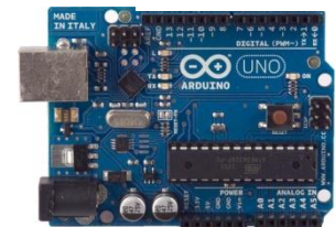
Figure 20: Image of an Arduino Uno microcontroller [1].
