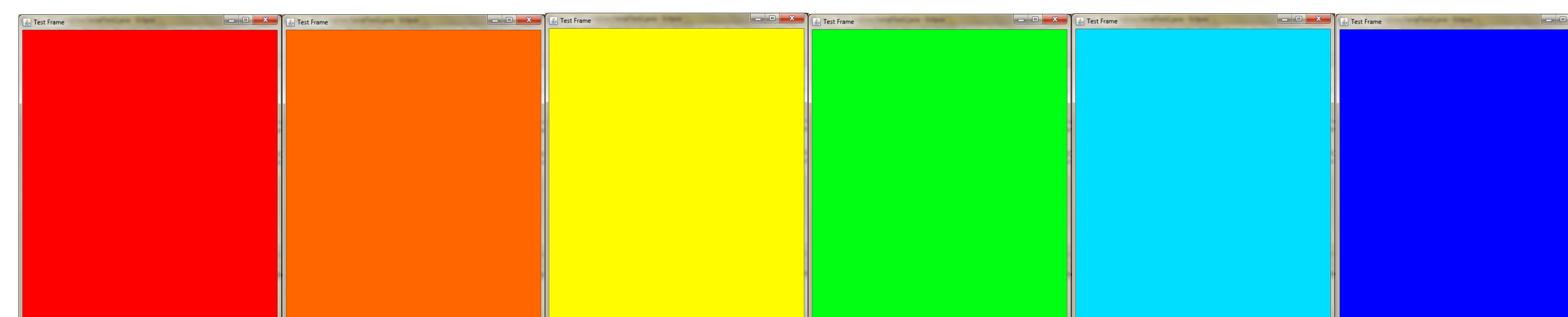
Figure 10: The color mapping algorithm is capable of displaying color values ranging from dark red to dark blue. A test frame displays the color corresponding to the voltage output of the sensor; red corresponds to a magnet directly over the sensor and dark blue to the sensor sensing no magnetic field.
