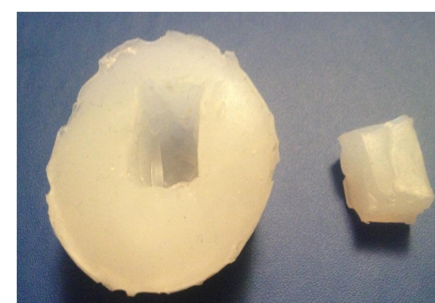
Figure 10: The sensor will be placed within a cavity and a plug of silicone will be placed on top of the sensor in order to secure the sensor in the uterine wall.
