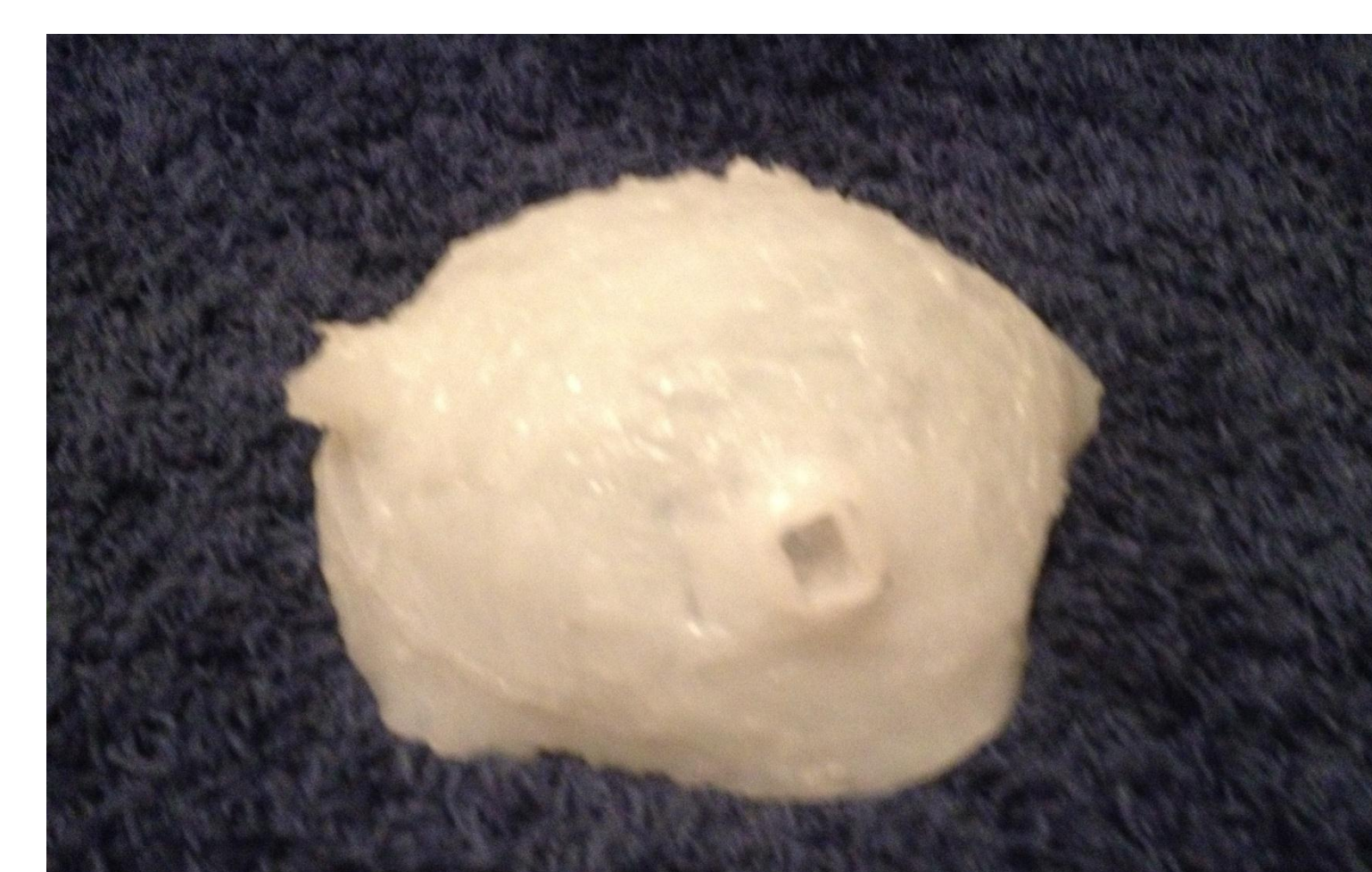
Figure 9: The upper 1/4 of the uterus with embedded magnets and open slots to house the sensors.
