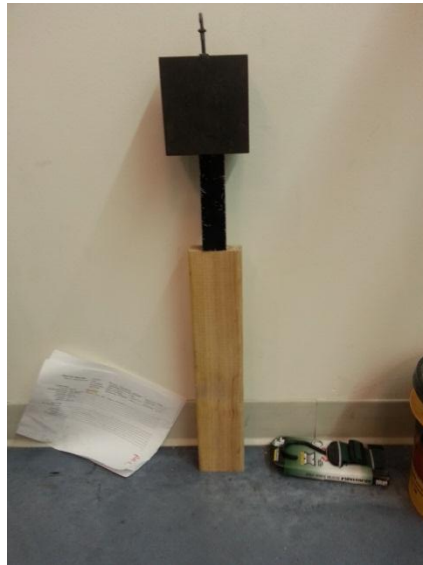
Figure 12: Axial compression test of prototype leg
