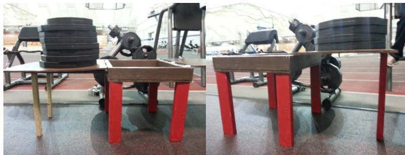
Figure 10: Testing of Prototype Components Backrest testing seen on left, and footrest testing seen on right.
