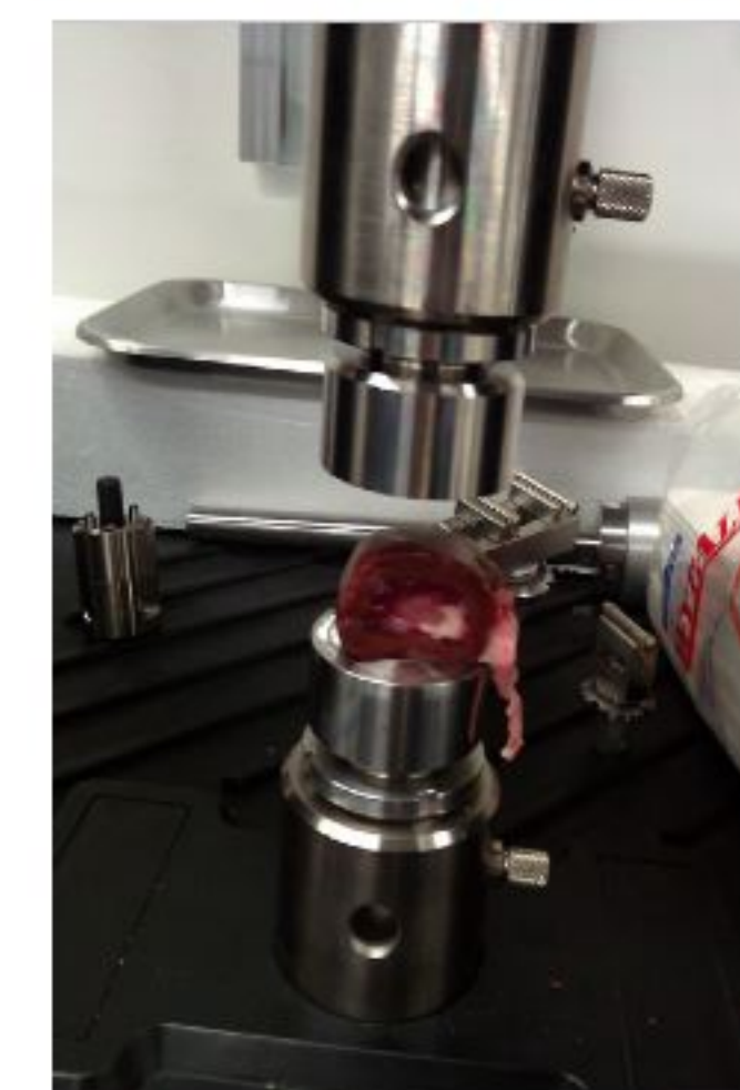
Figure 6. Image of compressive testing setup
