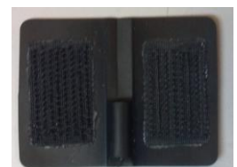
Figure 17: Example carbon/rubber electrode showing the Velcro placed on top of the electrode facilitating attachment to the electrode band.
