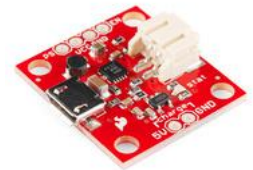
Figure 8: Power Cell – Lithium Polymer rechargeable battery charger and boost regulator. Capable of sourcing up to 600mA @ 5V. (sparkfun.com)
