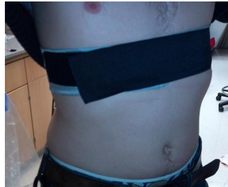
Figure 19: Electrode band prototype securely fastened on patient.
