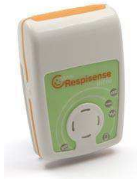
Figure 6: The RespiSense monitor attains mobility by clipping directly to an infant's diaper, and senses breaths by measuring pressure between a baby's belly and the waistband of the diaper (Infantrust, 2012).
