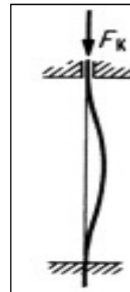
Figure 21: This image shows typical Euler buckling which has an axial force ( F_x ) causing elastic instability. 17
