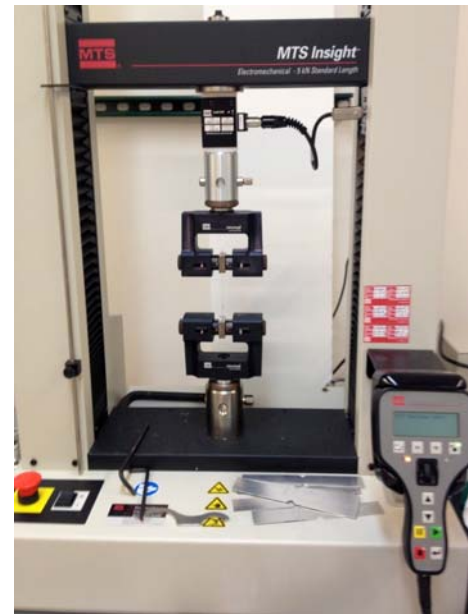
Figure 10: LLDPE sample loaded into the grips of the mechanical tester. Distance between the grips is controlled by the remote seen in the lower right hand corner. As the grips move apart, load and elongation data is recorded.
