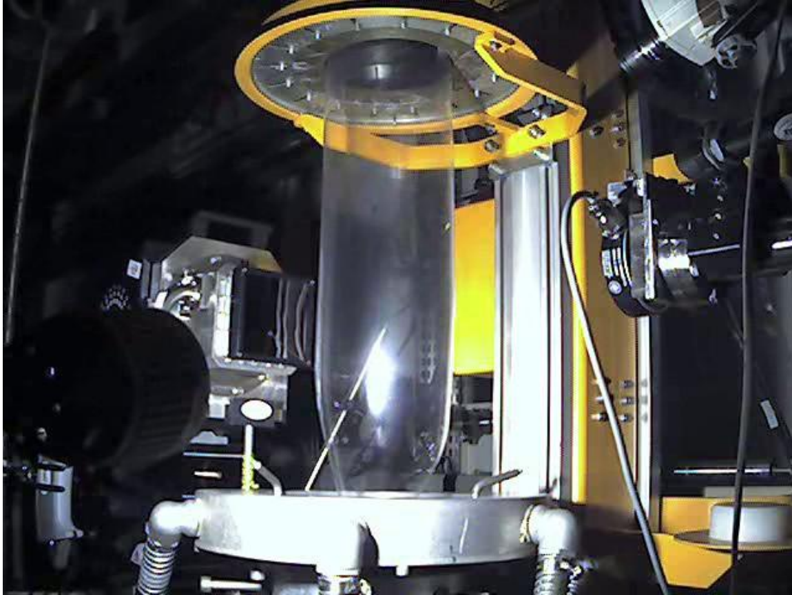
Figure 10: Film extrusion blower used to expand melted polymer into a flexible thin-film bag. http://www.esrf.eu/UsersAndScience/Experiments/CRG/BM26/pictures/BM26B/LDPE-film-blowing.jpg
