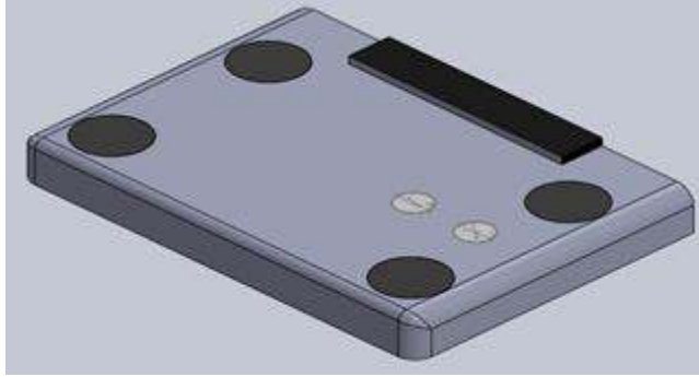
Figure 5: SolidWorks model depicting vibration feedback system. The vibrational motors can be seen, securely integrated within the framework of the board.
