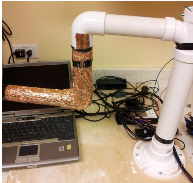
Figure 1: Client's current forearm model including the copper coated PVC pipe to represent the forearm and computer system which records temperature.
