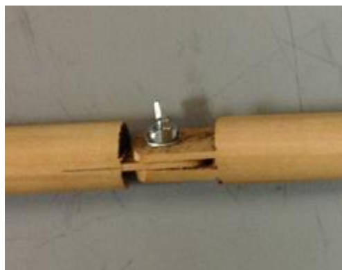
Figure 12: Three tab hinge system created out of wooden dowel
