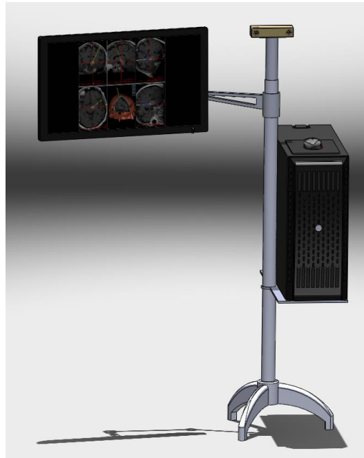
Figure 15: The spacing between the two cameras in the Bumblebee2 is predetermined. That and its internal processor aids in accurate 3D point tracking.
