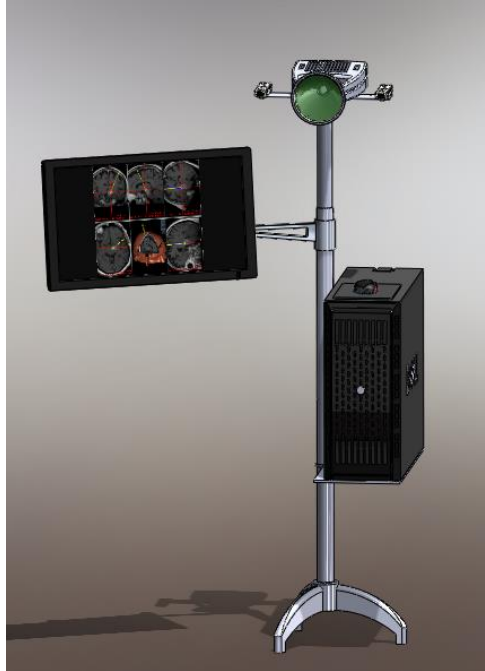
Figure 10: The Wii remotes require an IR lamp to increase accuracy. The entire setup, including the central computer and display unit, is shown. One Wii remote is placed on either side of the IR lamp at the top of the apparatus.
