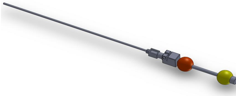
Figure 8: The Distal Series Tracker Rod attachment design
