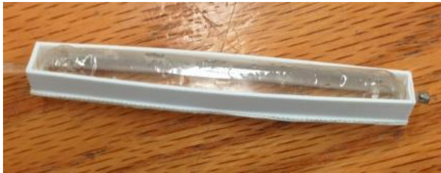
Figure 11. Catheter Design. The catheter design involves an expanding balloon to provide distraction.
