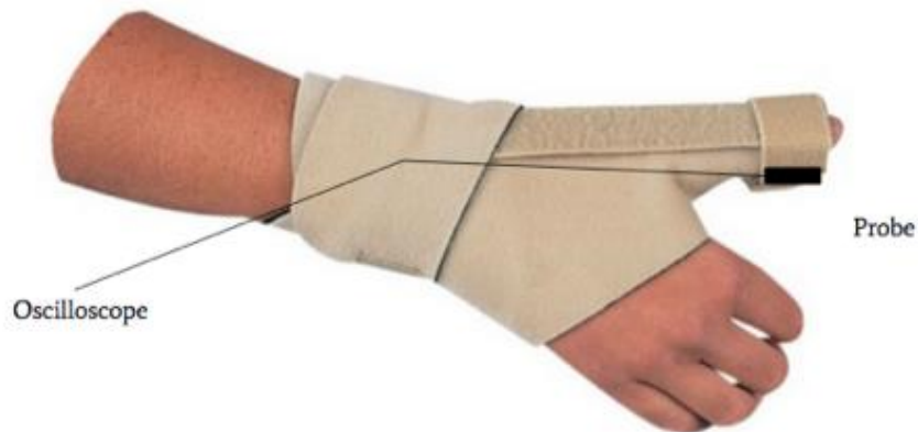
Figure 5. The splint design will wrap around the probe along with the wire connecting to the oscilloscope to further prevent any movement by the probe[8].
